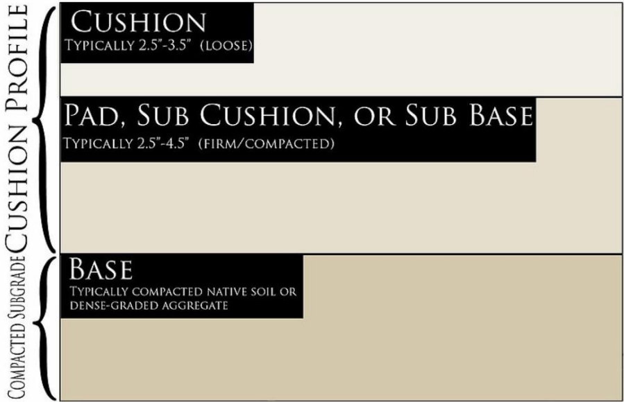
This diagram illustrates the recommended arena soil profile layers.
